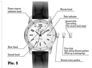
If your watch has a screwed-in crown, it should be unscrewed before manual winding, time and date setting. Do not forget to screw the crown back after the winding.
